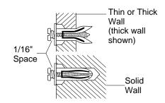
Figure 8 - Tightening Anchors
